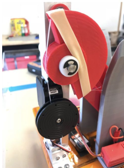
Fig. 4.2 - The completed lifting mechanism using two winch pulleys connected by fishing line and powered by a continuous servo motor.
